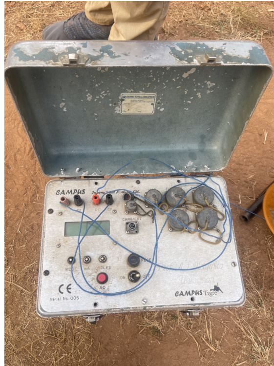
Figure 3. Resistivity meter used for the survey.
