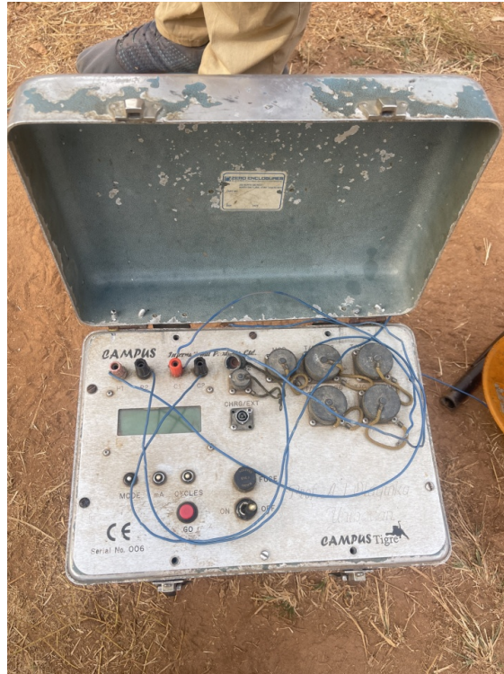
Figure 3. Resistivity meter used for the survey.
