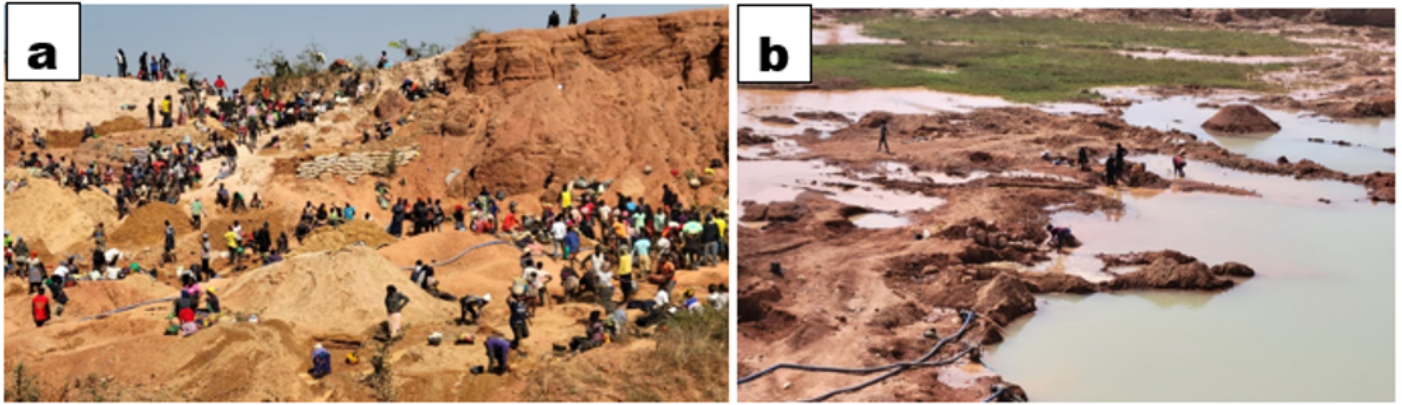
Figure 2. (a) Artisanal mining of tin from mine spoils in Du district of Jos south, Plateau state. (b) Mining and washing of tin from mine spoils into a water body at Rayfield.
